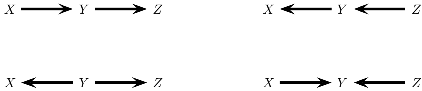
FIGURE 17.6. The first three DAG's have no colliders. The fourth DAG in the lower right corner has a collider at Y .
